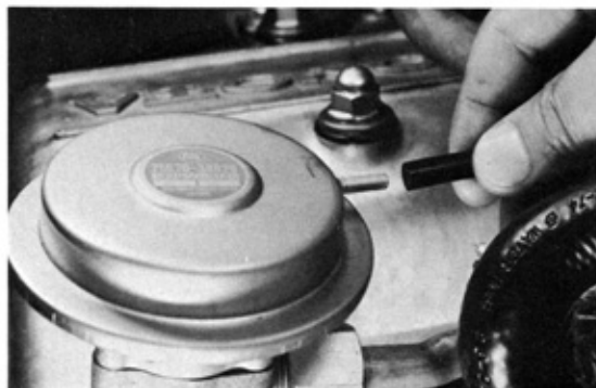
Fig. 2-32 Disconnect Hose From EGR Valve
